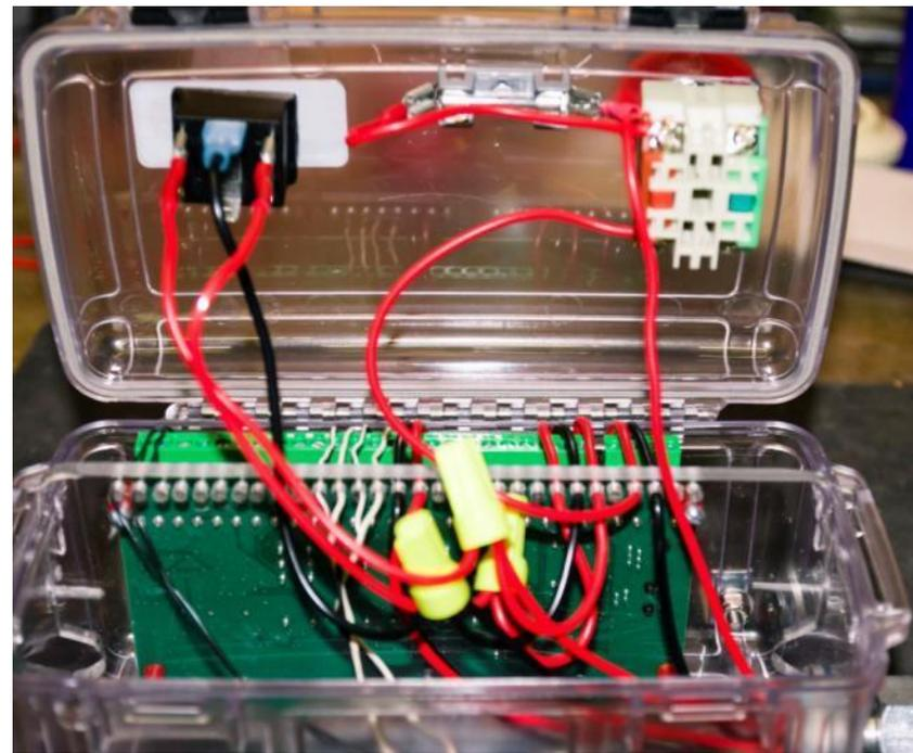
The hinged front of the box opens to allow easy access to the various connections. A series of 0.5 mm holes were drilled in the Lexan shelf to provide strain relief for the wires connected to the junction block of the MaxDome II card.
