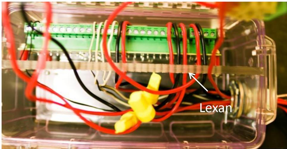
A piece of  $\frac{1}{4}$  inch Lexan was cut to fit the inside of the box and serves as the mounting platform for the interface card. It is held in place with stainless steel screws on the sides and back.
