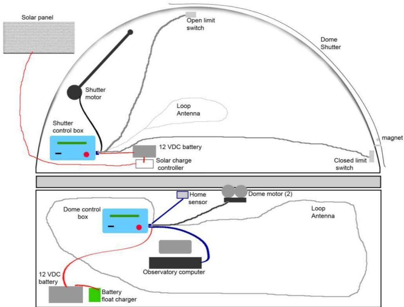
An interface box riding on the dome holds the MaxDome II card that controls the reversible shutter motor. It is powered by a small 12vdc battery which is continually recharged by a solar panel. Open & closed limit switches keep track of where the shutter is. A magnetic inductance loop antenna communicates with a larger loop antenna connected to the dome controller. The dome controller also has a MaxDome II card that controls rotation and receives commands from the observatory PC.
