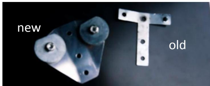
Here's how I solved the problem with the poorly fitting pulleys. The guides on the pulleys are PVC and will tolerate a bit of heating to reshape them. I used a hobby style heat gun to gently warm the PVC.
