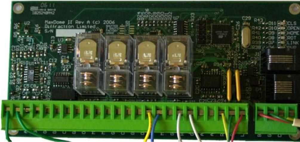
For control of the shutter I used the MaxDome II interface card from Cyanogen. This is the same card used for controlling rotation of the dome, but configured to operate the shutter. It consists of a series of relays along with connections for open and closed switches, a manual operation switch, and a magnetic inductance antenna for communication with the rotation controller.
