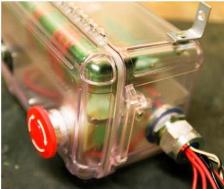
A  $\frac{3}{4}$  inch lead connector with compression fitting acts as a port for the power, switch, and antenna lines that connect to the MaxDome II card. A simple right angle bracket mounts to the top of the box for attachment to the dome.
