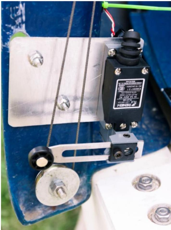
I opted to use two different types of limit switches. For the “closed” switch I used a mechanical limit switch (left) with an adjustable arm. A small piece of aluminum angle mounted on the front shutter contacts the arm as the shutter is almost closed. Because of slack in the pulley system, the shutter tends to fall about an inch when power is removed; the mechanical limit switch arm remains in contact with the shutter throughout this extra movement.
