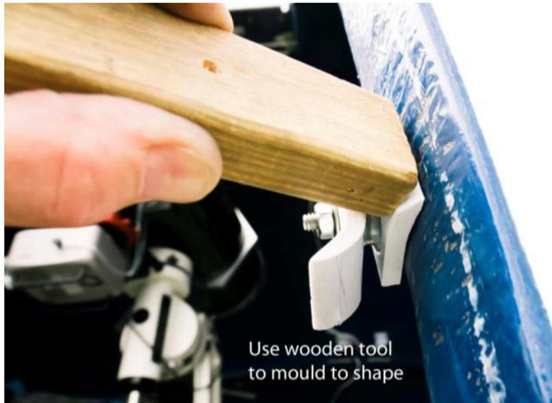
Then using a wood block I pressed the guide to match the shape of the shutter flange and held until the PVC cooled. If done carefully this makes each pulley have a custom fit and does not interfere with the movement of the pulley. The same technique can be used on the curved guides to form them to allow the shutter mechanisms to clear.
