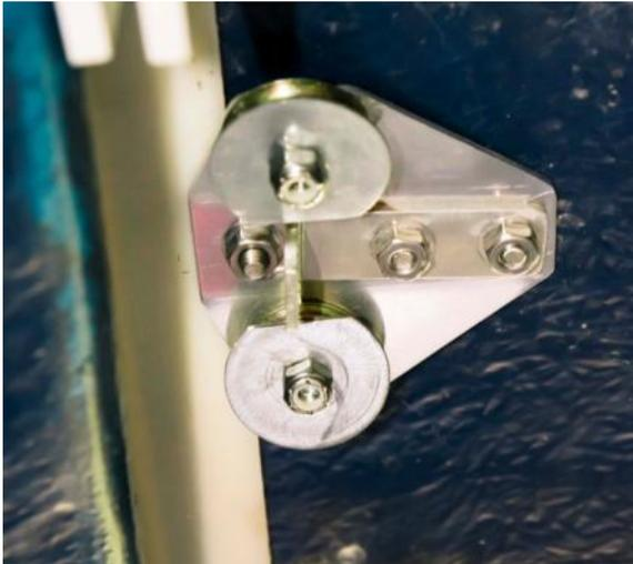
The image at the left shows the replacement pulley assembly mounted in place at the correct distance from the shutter flange. The guide for the shutter locking mechanism is installed on top of the pulley assembly.
