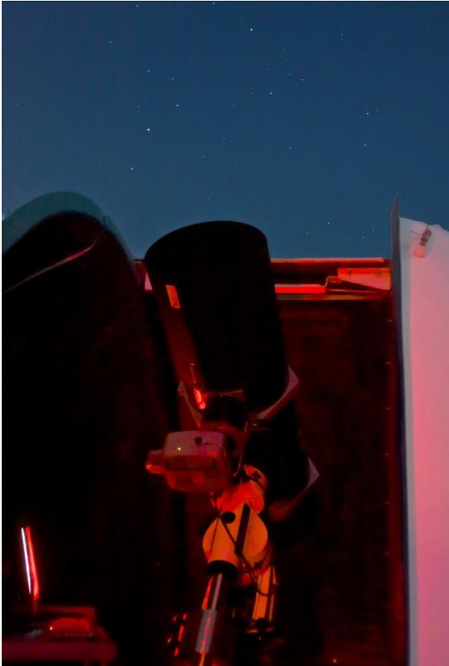
The automated shutter now allows unattended imaging. I use the ASCOM dome control panel, or the dome control routines incorporated into MaximDL to open and close the shutter, and to park the dome. The dome is routinely slaved to the mount.
