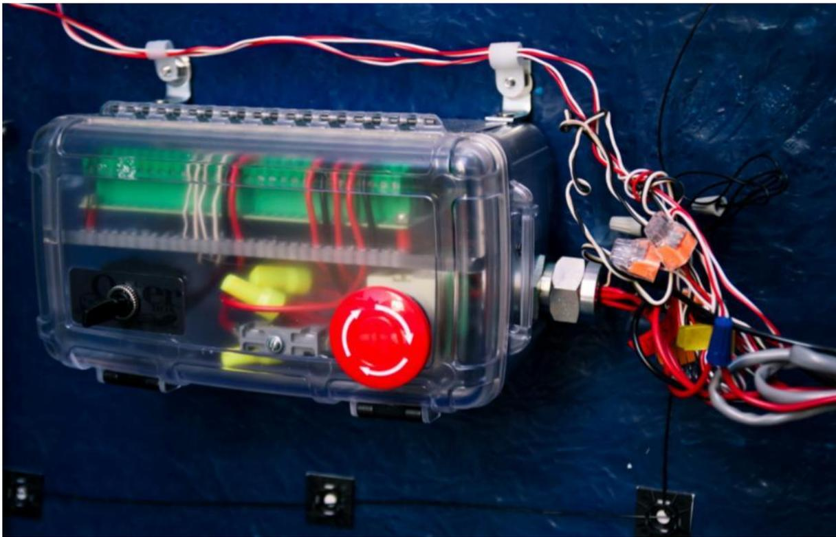
The image at the left shows the interface box with MaxDome II card mounted inside. The angle brackets at the top are used with stainless steel flat head screws to mount the box near the bottom of the rear shutter. A more sophisticated interface box with additional relays and a soft-start card for the motor (Chris Erickson, Summit Kinetics) will be installed in the future.
