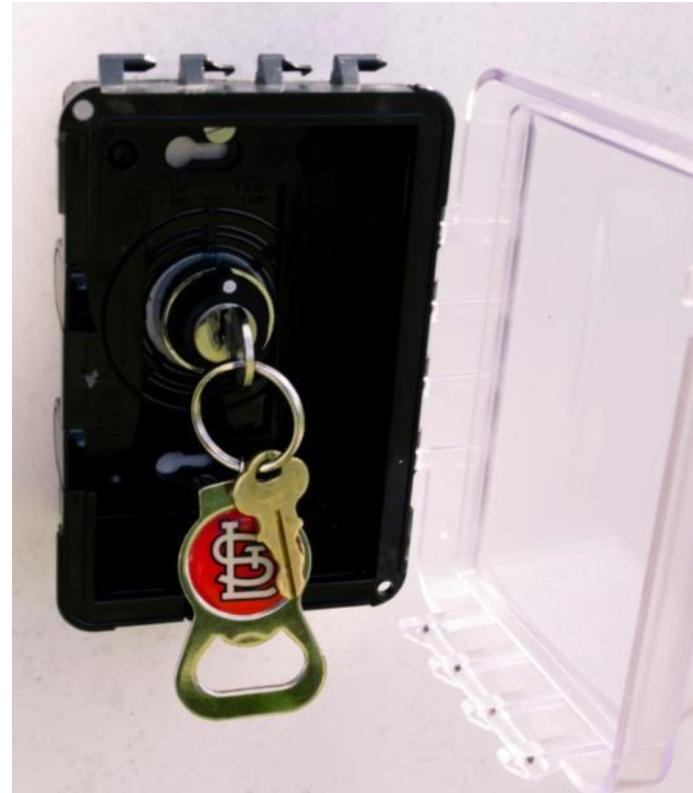
In order to open or close the shutter manually, I installed a key-operated momentary DPDT switch. This switch is wired in parallel with the manual switch mounted on the interface box. The key switch is mounted in a convenient location next to the shutter in a weather-proof box. The key is held in the appropriate position (open or close) until the shutter reaches the end of its travel and the limit switches remove power.
